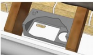
Eaves S Brick resting on the soffit
