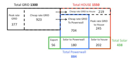
Estimated Power Flows for Nov, Dec, Jan with 5kW PV and Tesla Powerwall in 'Cost Saving' mode.
